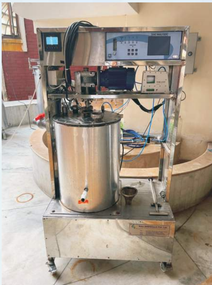
50-L Anaerobic digester at SSS-NIBE
