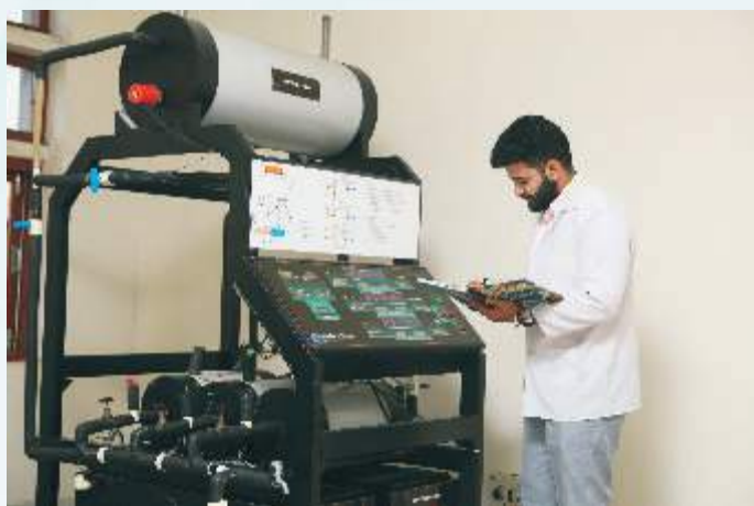
Researchers working on the Thermal Energy Storage and Solar PV Training & Research System
